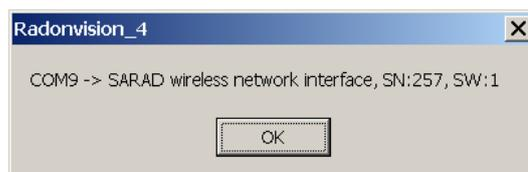
The adapter will be automatically detected during the port check sequence and can be accessed via the assigned COM port index.
