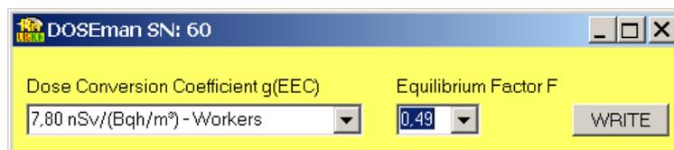
Because any dose calculation is based on the Radon exposure respectively the Radon daughter products, the Equilibrium Factor F has to be estimated if the Radon exposure (concentration) was measured in case of the DOSEman. The Equilibrium Factor defines the assumed ratio between Radon daughter products and Radon gas. If the real conditions are not known from earlier investigations it should be set to 0.5 what is a reasonable value for the most places.
