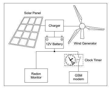
30% of the stated peak power depending on the place of installation. The battery capacity has to be large enough to ensure the power supply over longer cloudy periods.
