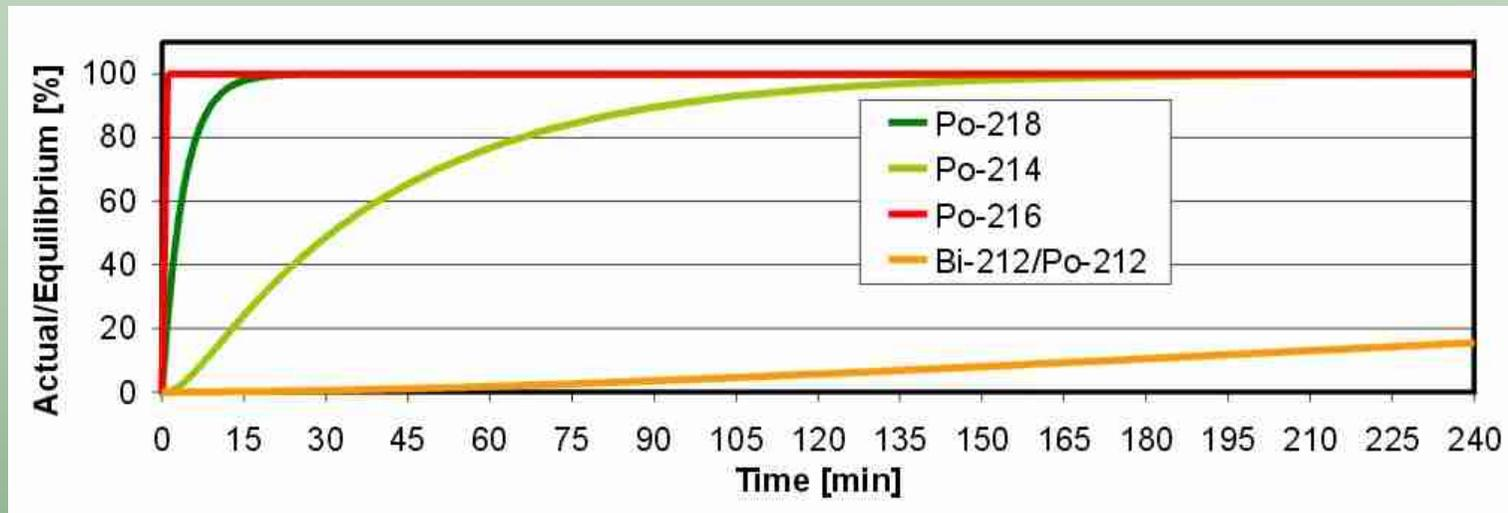
Radon calculation based either on **Po-218** only (**Fast Mode**) or on sum of **Po-218** and **Po-214** (**Slow Mode**)
