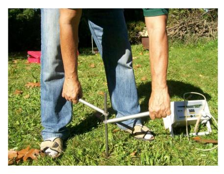
Pull out the hollow probe after the measurement with 2 small retractors.
