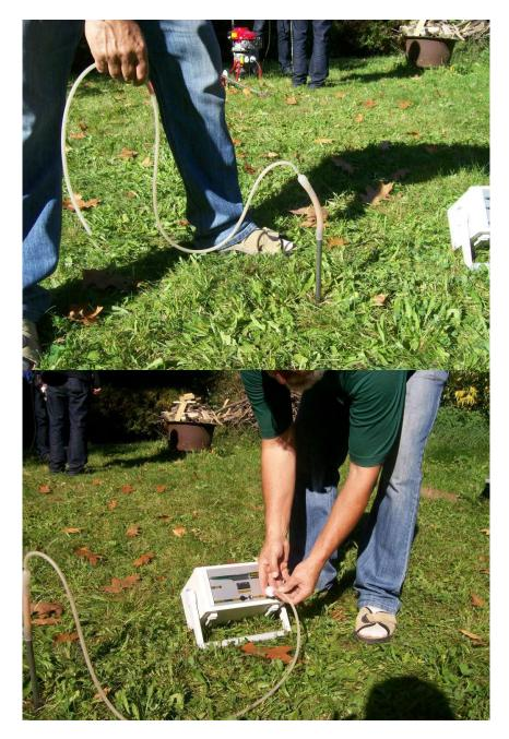
Connect the radon measurement instrument (for instance RTM 1688-2) and start the measurement cycle (integration time 5 minutes, measurement time min. 15 minutes).
