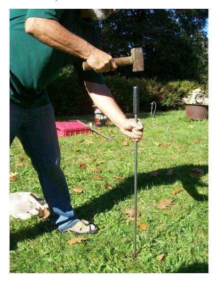
Punch the hollow probes into the ground.
