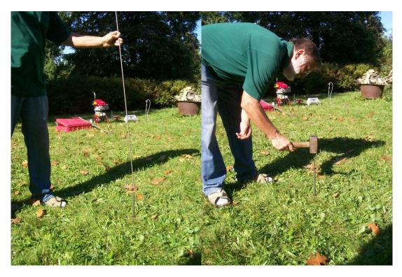
Put the punch wire inside the hollow probe, so the sharp tip will be pushed out and a small sampling volume is formed.
