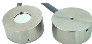
In a large number of OEM applications, Alpha- and Beta radiation detection units are required which are providing high noise immunity, simple interfacing and small form factors. The modules MOD-01/03 and MOD-01/04 offer a perfect solution for that. They combine a light-shielded, ion-implanted detector, a charge sensitive preamplifier and a shaping amplifier inside a rugged and small enclosure. Several detector sizes are available.
