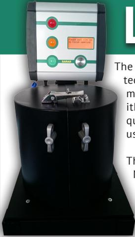
The Lab Scout is a very easy to operate instrument to detect and quantify natural and artificial radionuclides in material samples. For standard operation procedure neither a computer nor special skills of the operator are required. On the other hand, the instrument can still be used as a flexible and powerful tool in the laboratory.
