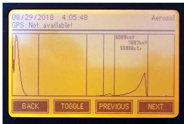
The typical example of a Radon spectrum shown at the picture above contains four significant peaks as a maximum. The following table points out some criteria for the spectrum shape with respect to the peak area, peak shape and peak position:
