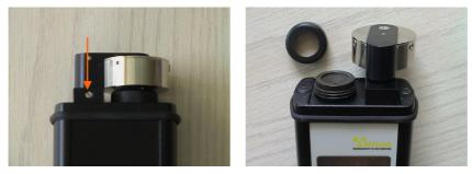
away the pivot arm backwards for free filter access. Unscrew the filter nut anti-clockwise and remove the old filter. The measurement head must not be turned around for several times because the connection wires could become damaged! Do not
