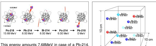
This energy amounts 7.68MeV in case of a Pb-214, Bi-214 or Po-214 atom while Po-218 will emit 13.68MeV (6MeV as Po-218 and additional
