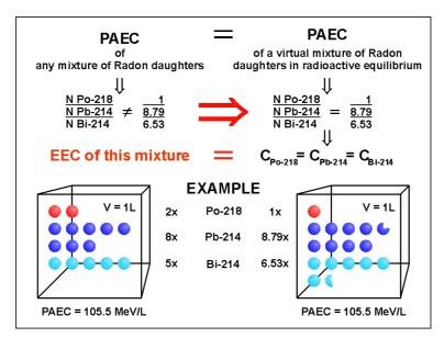
This causes a linear relationship between the measured PAEC and the resulting activity concentration which is called Equilibrium Equivalent Concentration (EEC).
