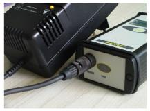
To charge the battery, the charger has to be plugged to the mains power line firstly. After that, the cable can be connected to the charge receptacle of the DOSEman-PRO. The red LED lamp will blink for a few Seconds (battery check) and afterwards light permanently. At the end of the recharging process, the LED lamp switches from red to green light.
