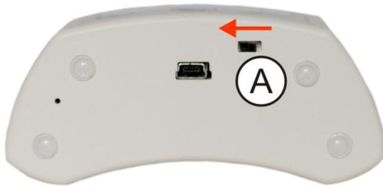
Fig. 3. – Set the sliding switch (A) to the left position (no sampling) and wait until the instrument enters standby mode (display off).
