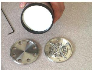
Take away the inner sealing plate and the outer stabilisation grid. Now, the membrane is accessible and can be removed. Do not use sharp edged tools which could damage the sealing surfaces.
