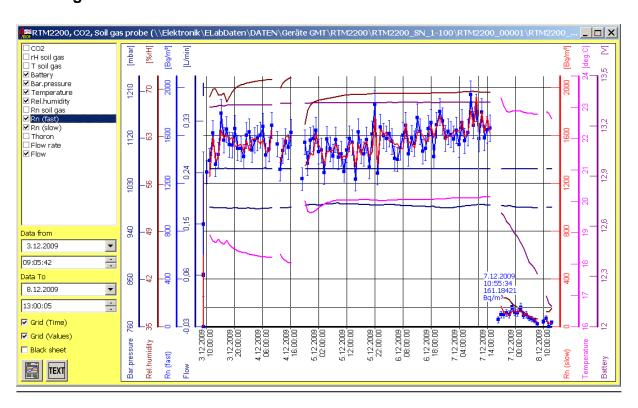
The diagram window contains all functions which are required for data visualisation and output. It is opened after reading data from an instrument or loading a data file. The track selection box in the left upper part of the window shows a list of all data tracks which have been acquired by the instrument. If the small box left beside the track name is checked, the time distribution is shown in the diagram, assumed that some data of the track is present within the selected measurement period.
