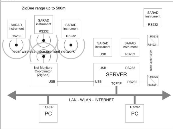
The operational software for DACM based instruments contains a complete solution for TCP/IP based communication with the most of SARAD instruments. The Implementation is very easy and does not require special skills in the IT field. If the available network structure of an organisation shall be used, the assistance of the responsible network administrator may be required.
