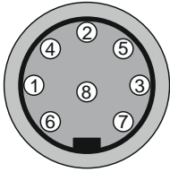
Socket „AUX1“ (Binder Series 680 – DIN 8-pin), front view of the socket
