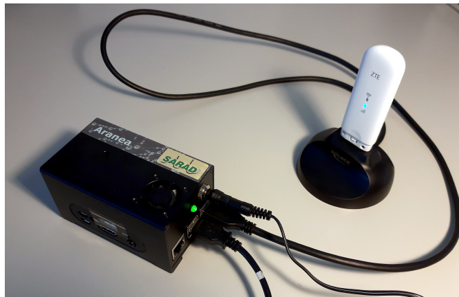
Figure 2.2: Aranea LTE with LTE modem connected via the USB extension. The USB extension may differ from the one shown in the photo.
