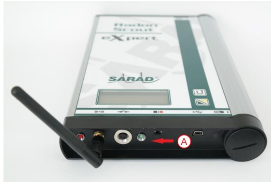
Fig. 3. – Set the sliding switch (A) to the left position (no sampling) and wait until the instrument enters in standby mode (display off).
