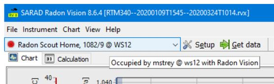
Figure 6.4.: Display of the reserving user with host name and application program
