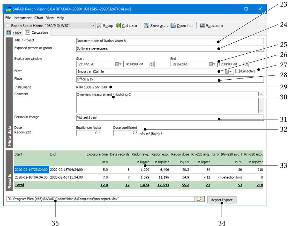
Figure 5.2.: Operating and display elements in the *Calculation* tab
