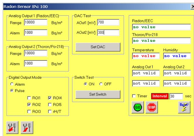
Figure 5.6.: Additional setting options for the *Analog Sensors*
