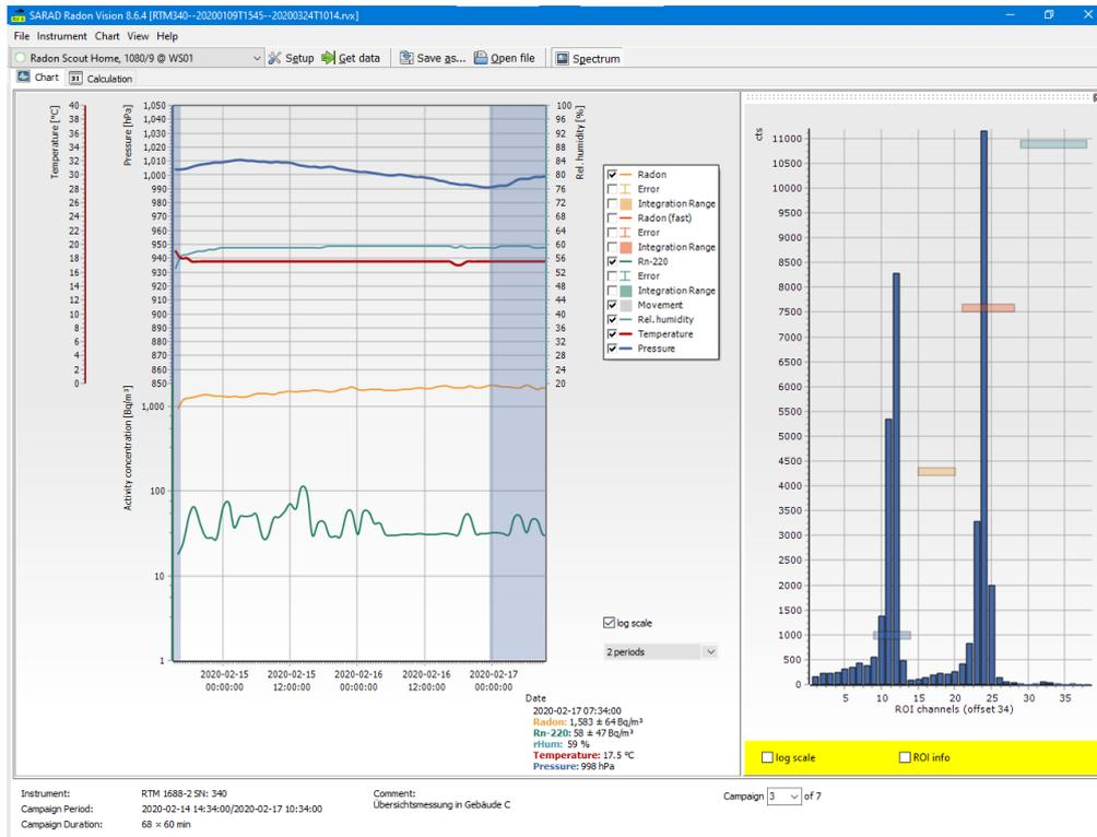
Figure 5.8.: Docked spectrum display; logarithmic scaling in the line diagram and smoothing with a moving average over two periods. The ROI information in the spectrum histogram is switched off to make the ROI limits more visible.
