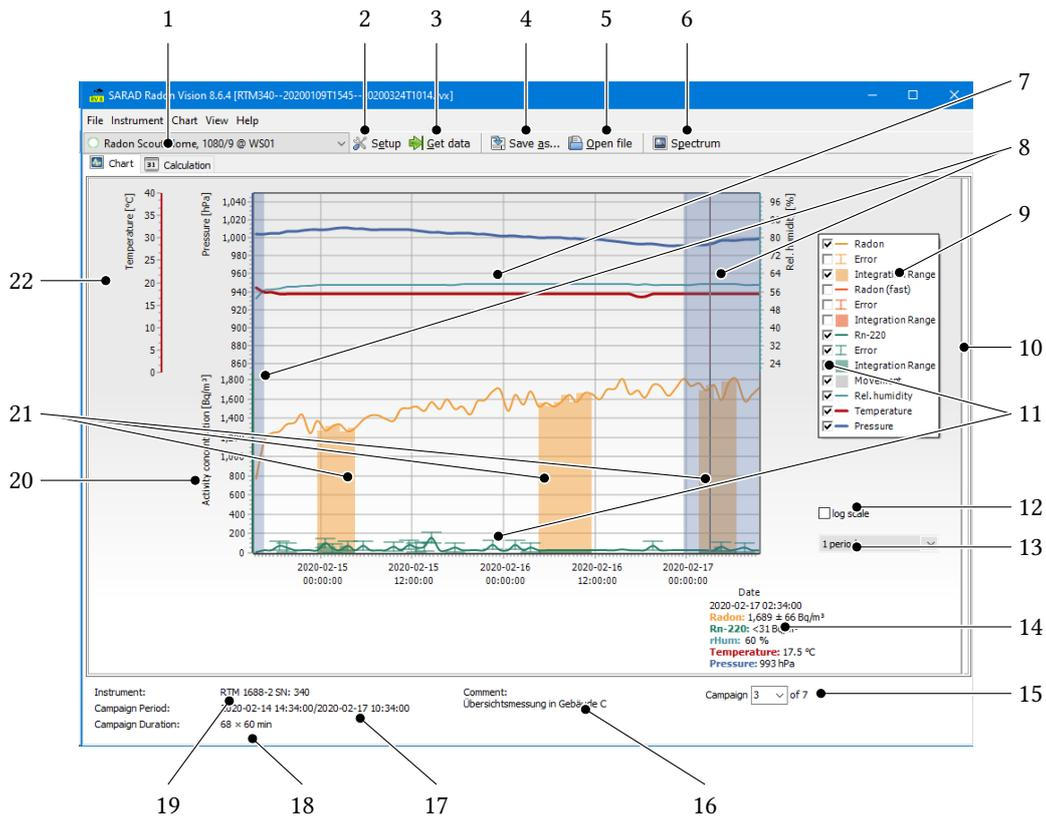
Figure 5.1.: Operating and display elements in the *Chart* tab
