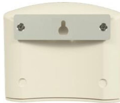
Figure 7 Smart Radon Sensor with the mounting clip
