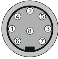
Socket „AUX2“ (Binder Series 680 – DIN 8-pin), front view of the socket
