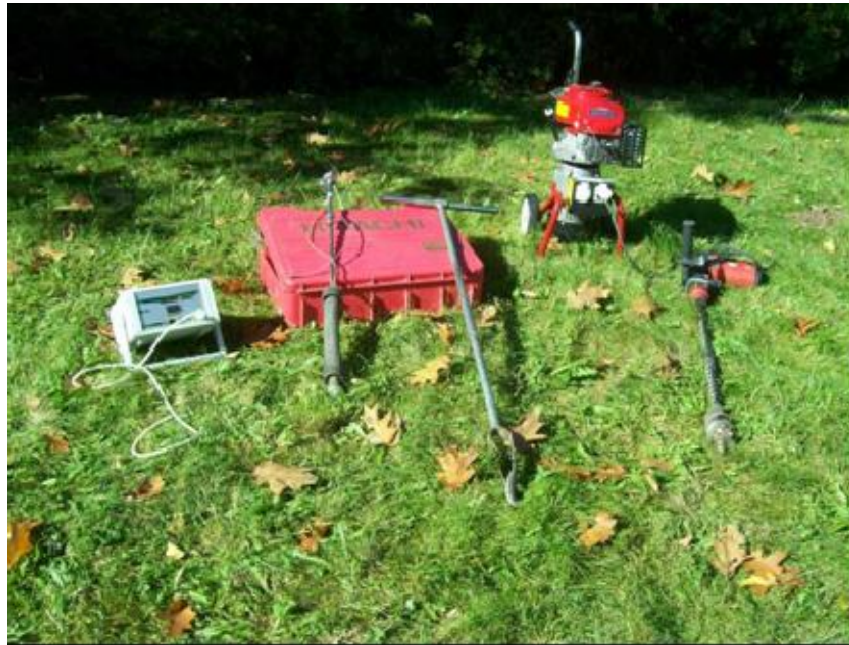
Hand drilling set with gravel head, packer probe alternative machine drill and generator
